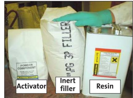
5 litre can of resin, 15 kg of inert filler and activator in carton.
